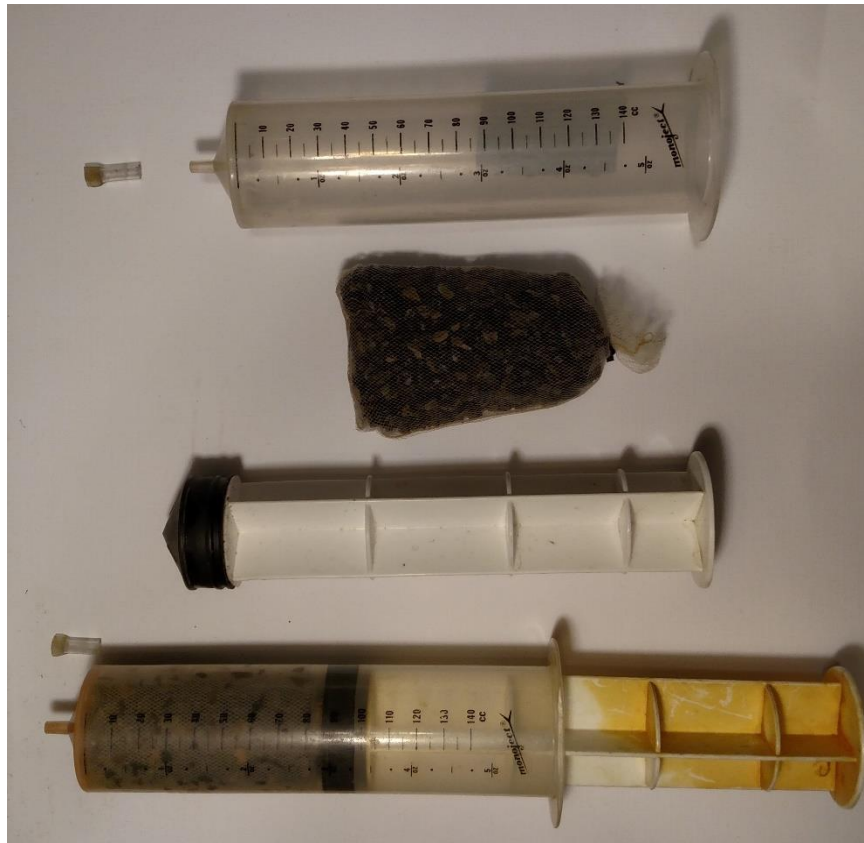
Figure 1 The standard composition of an Alkast is a 140 mL syringe, a mesh bag with material, and an airtight cap.
